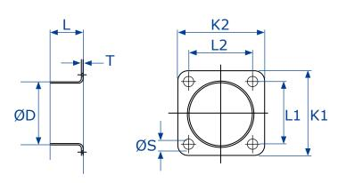
Outlet connector for HAPROVENT M Model S
