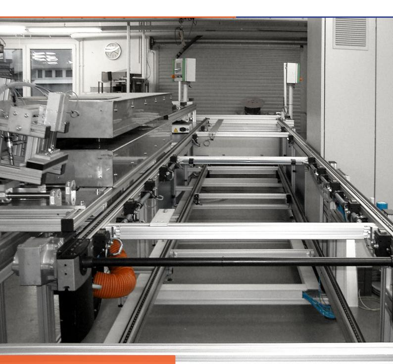
On the far left of the picture you can see the crimping unit, and behind it the shrink tunnel. The switch cabinet is on the right and the controls can be seen in the background.
